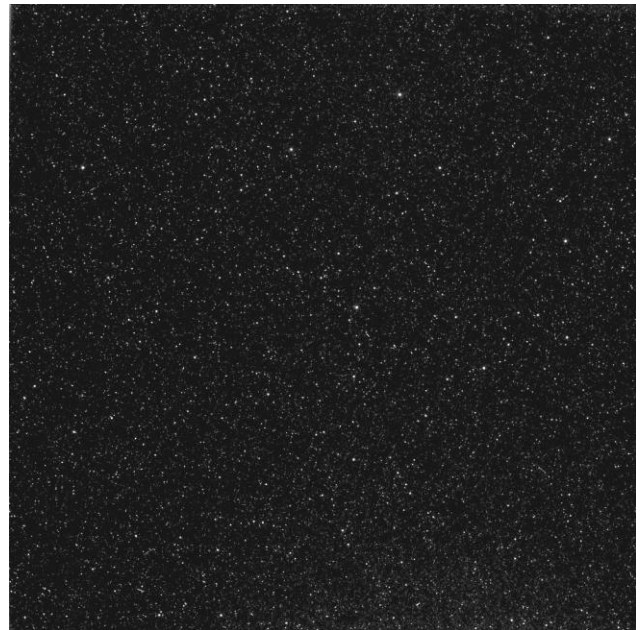
Figure 38. First light with the WAC, 5 s exposure with the red broad band filter. The WAC image contains the NAC view at the centre 1/5 FOV (horizontally mirrored).
