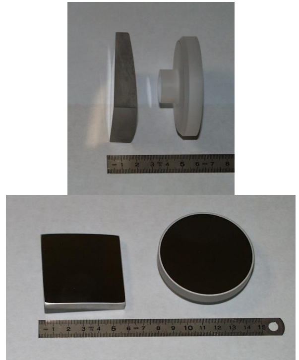
Figure 11. WAC mirror blanks M1 (bottom) and M2 (top).
