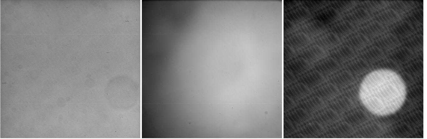
**Fig. 4.** Example of ground flat-field frames used to calibrate the images. *Left:* flat-fields for NAC orange images. *Center:* flat-field for WAC OI images. *Right:* Flat-field for WAC OH images. In this last image a pinhole is clearly visible.
