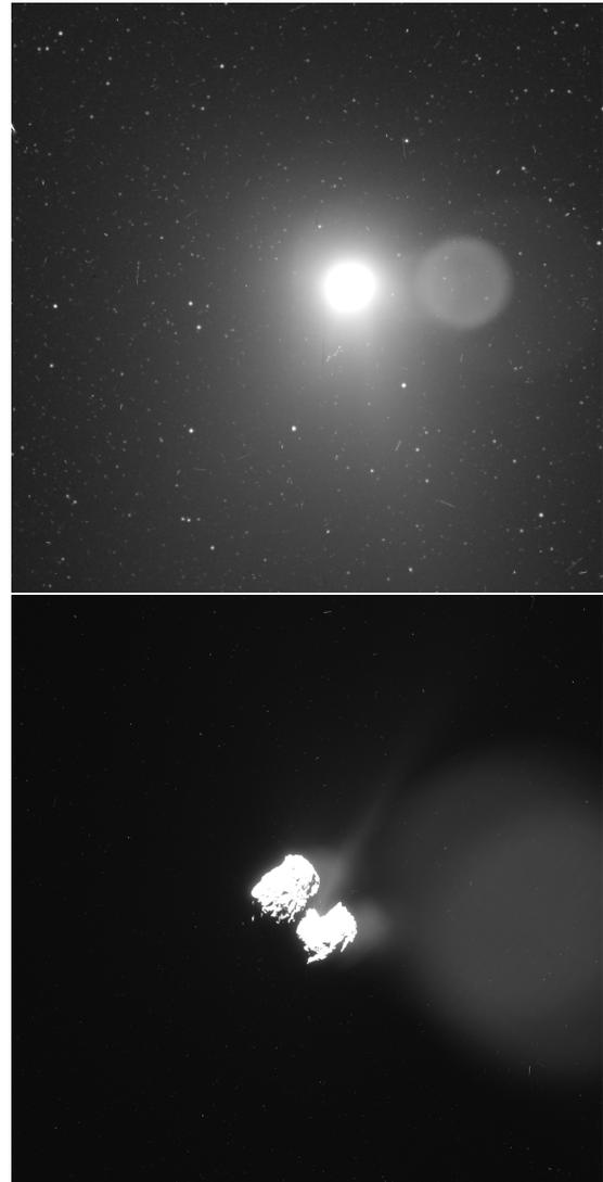
**Fig. 8.** *Top panel:* image of 67P acquired on July 25, 2014. A ghost is clearly visible on the right-hand side of the image. *Bottom panel:* image acquired on August 8, 2014. The ghost is in the same position as in the top panel and it is blending with the coma, creating artificial structures.
