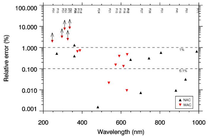
**Fig. 6.** Relative errors of the absolute calibration coefficients versus wavelength. The WAC UV filters that are affected by pinholes, which effectively decrease the accuracy of the radiometric calibration, are marked by a black arrow to indicate that the relative error is larger than the value shown.
