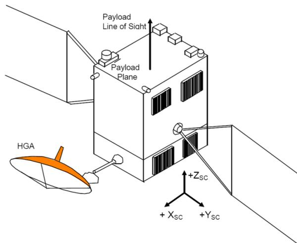
**Figure 6: The Rosetta spacecraft coordinate frame (S/C-COORDS) definition**
