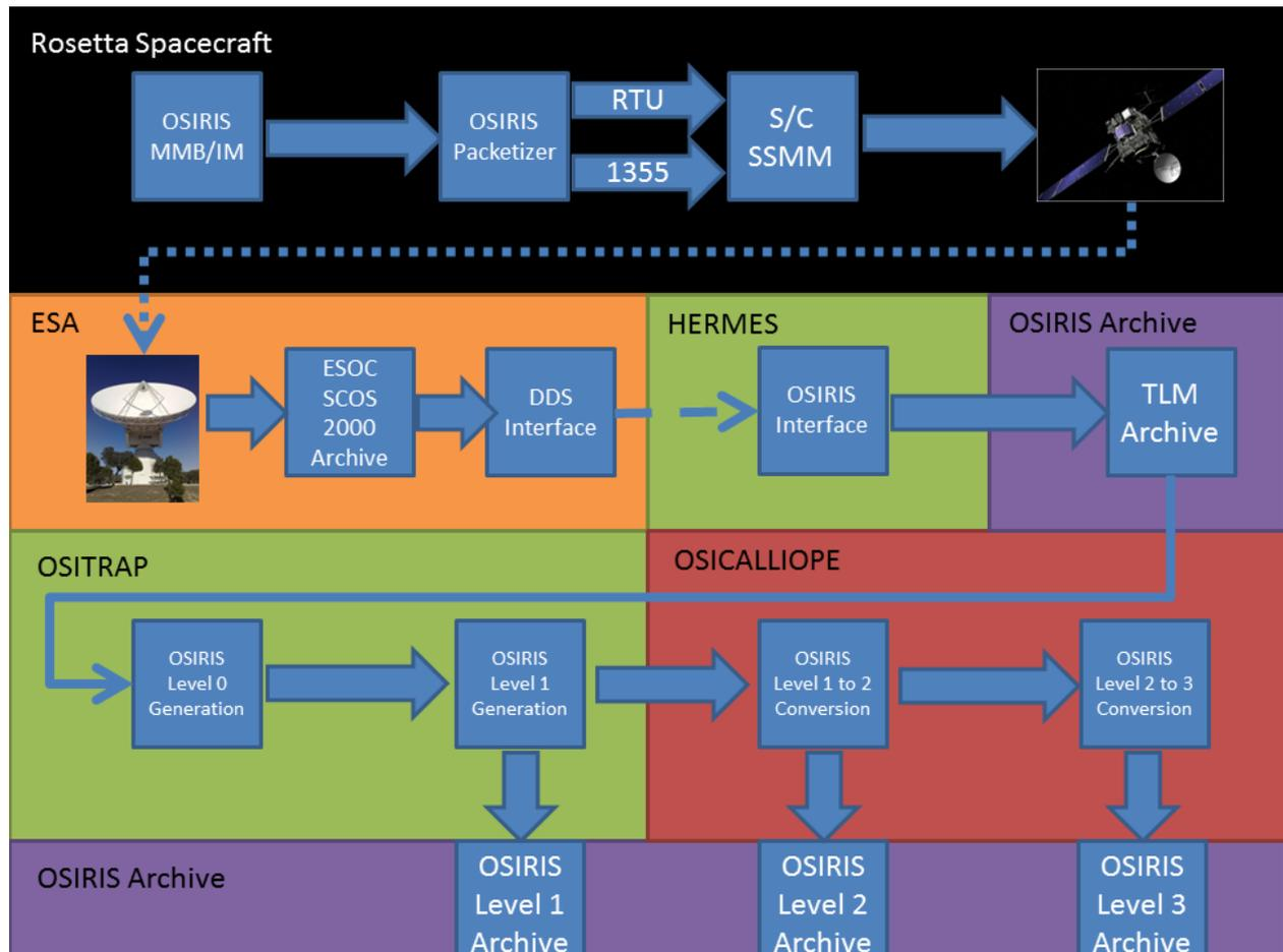
**Figure 3: The OSIRIS data and processing flow**
