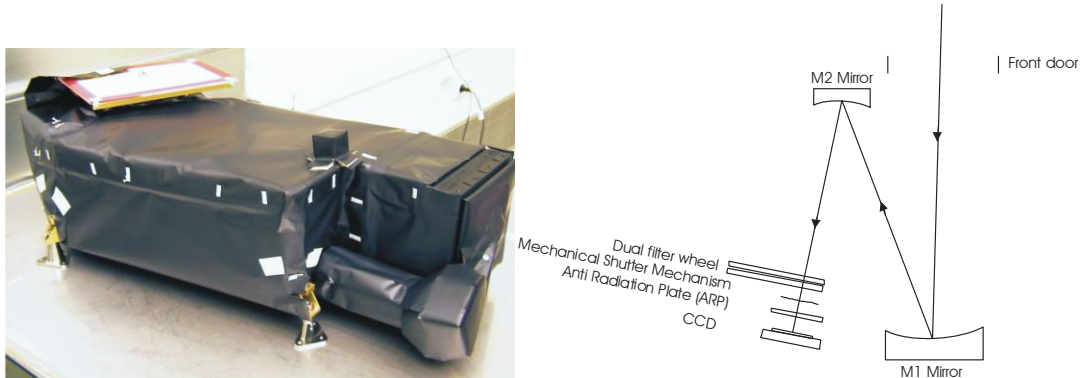
Figure 3 (left) The OSIRIS WAC flight unit in the lab. (right) The WAC Optical path
