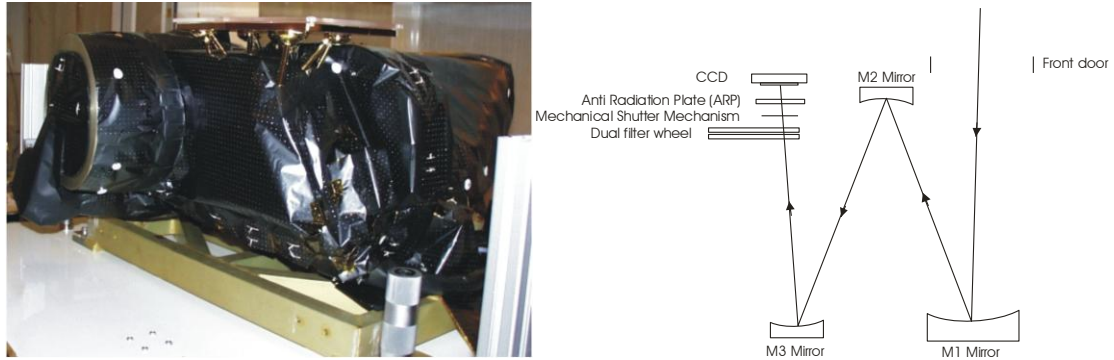
Figure 1 (right) The OSIRIS NAC flight unit in the lab. (left) The NAC Optical path
