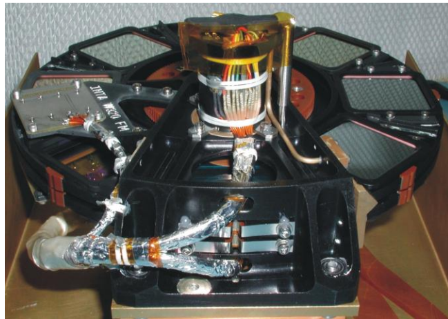
Figure 2 The OSIRIS dual filter wheel mechanism
