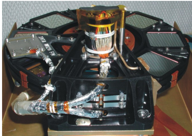
Figure 2 The OSIRIS dual filter wheel mechanism
