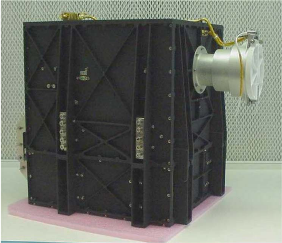
Figure 4. The instrument with the funnel cover closed in launch configuration.
