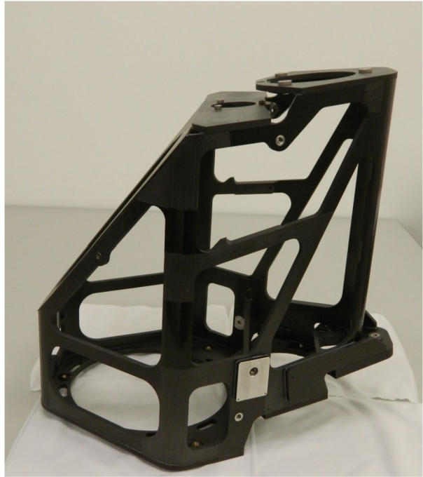
Fig. 6 The CFRP structure of the telescope prior to mounting of the mirrors
