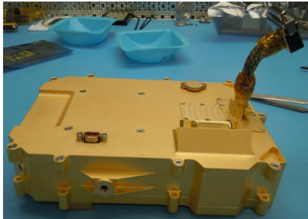
Fig. 9 The Proximity Electronics housing containing the PE board for driving the FPA. The board is similar to that used on SIMBIO-SYS but with small modifications to the connector positioning so that the box could be mounted inside the rotation bearing. The box is roughly 20 cm in length
