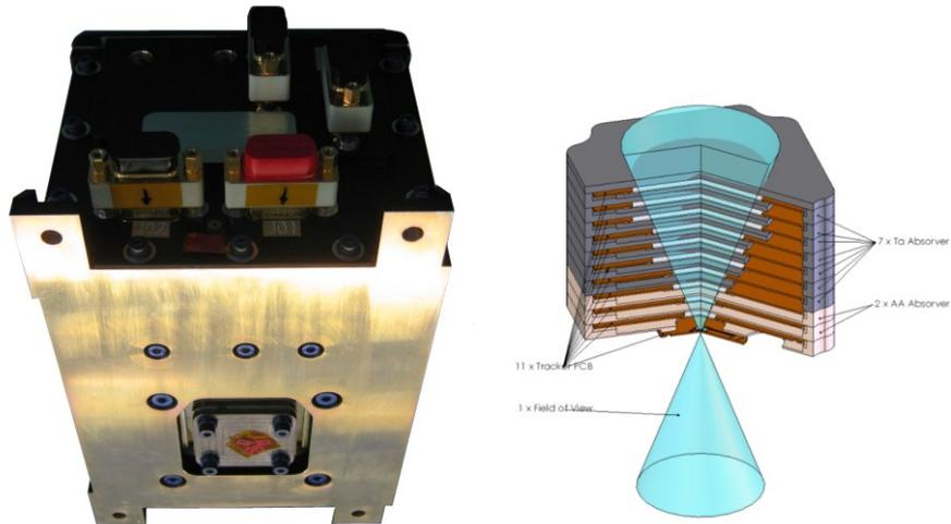
**Figure 1 (a) BERM flight unit and (b) Frontend/Detector stack schematic overview**
