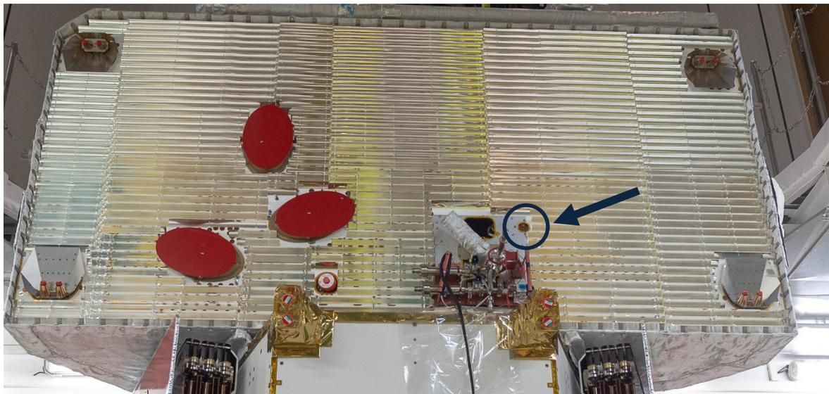
**Figure 2 Location of the BERM aperture on the spacecraft radiator panel**
