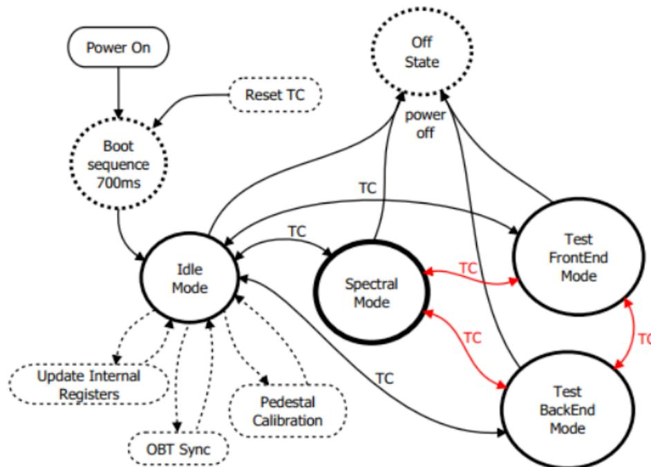
**Figure 3 BERM Mode Transition Diagram**
