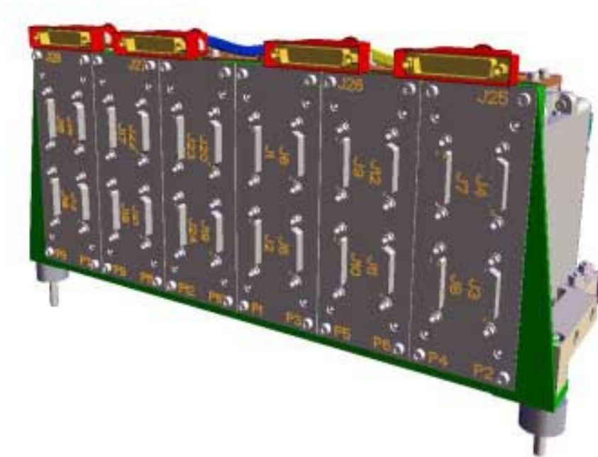
Figure 5.4-4 : SPIRE Photometer JFET rack external configuration
