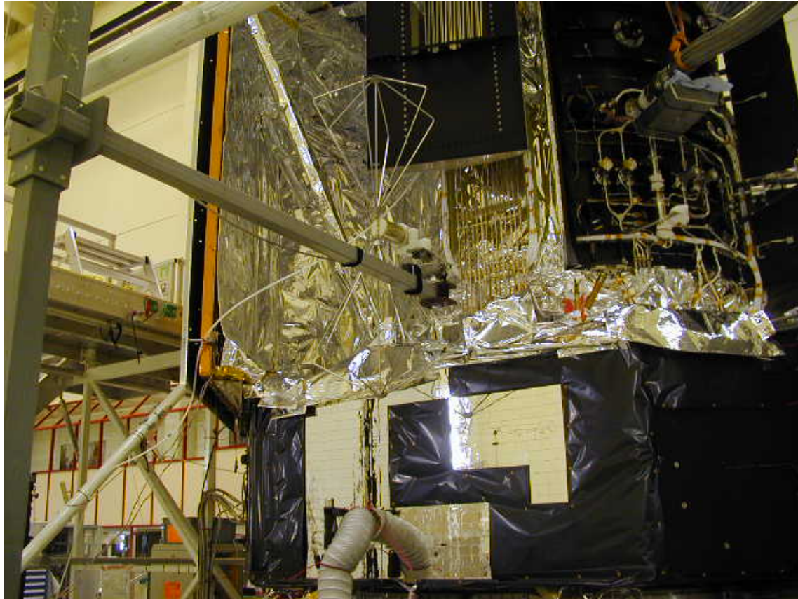
HIFI position EM 30 MHz to 200 MHz Vertical Polarisation
