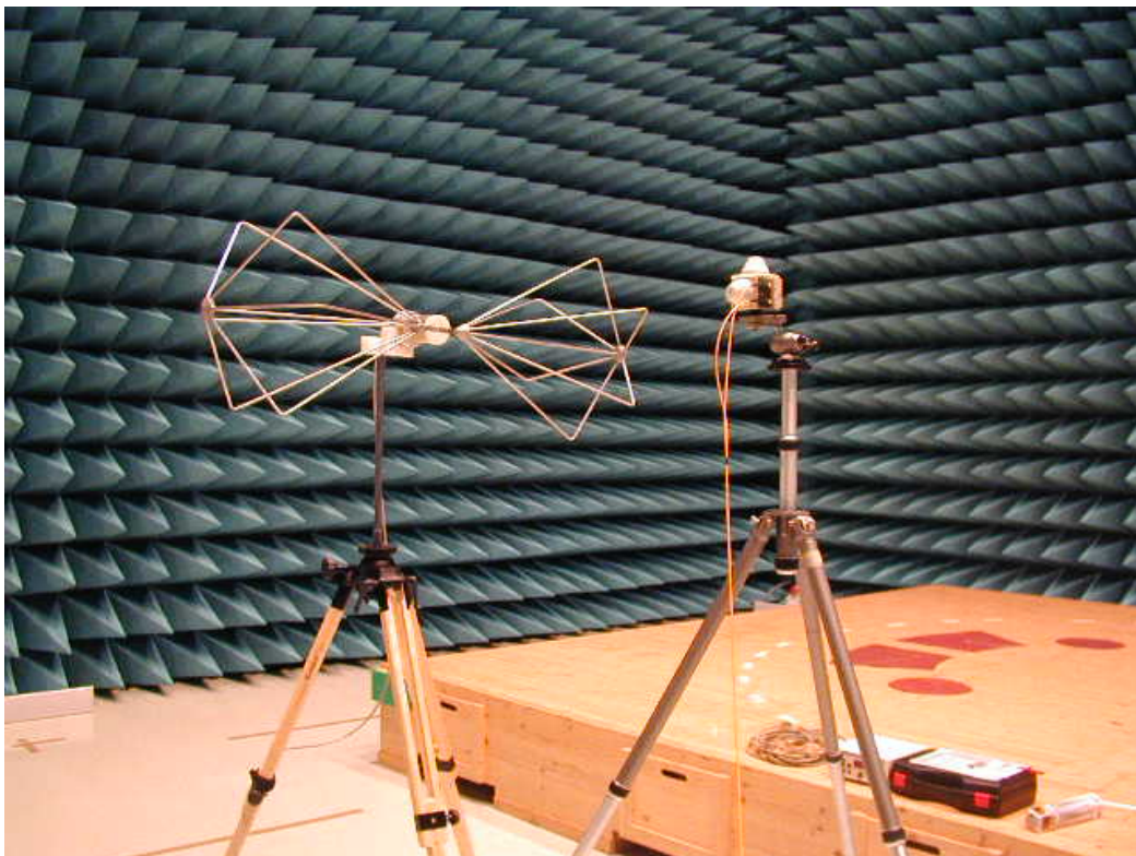
RS field calibration 10-100MHz Horizontal Polarisation >1 V/m at 1 meter distance and 2 meter above floor
