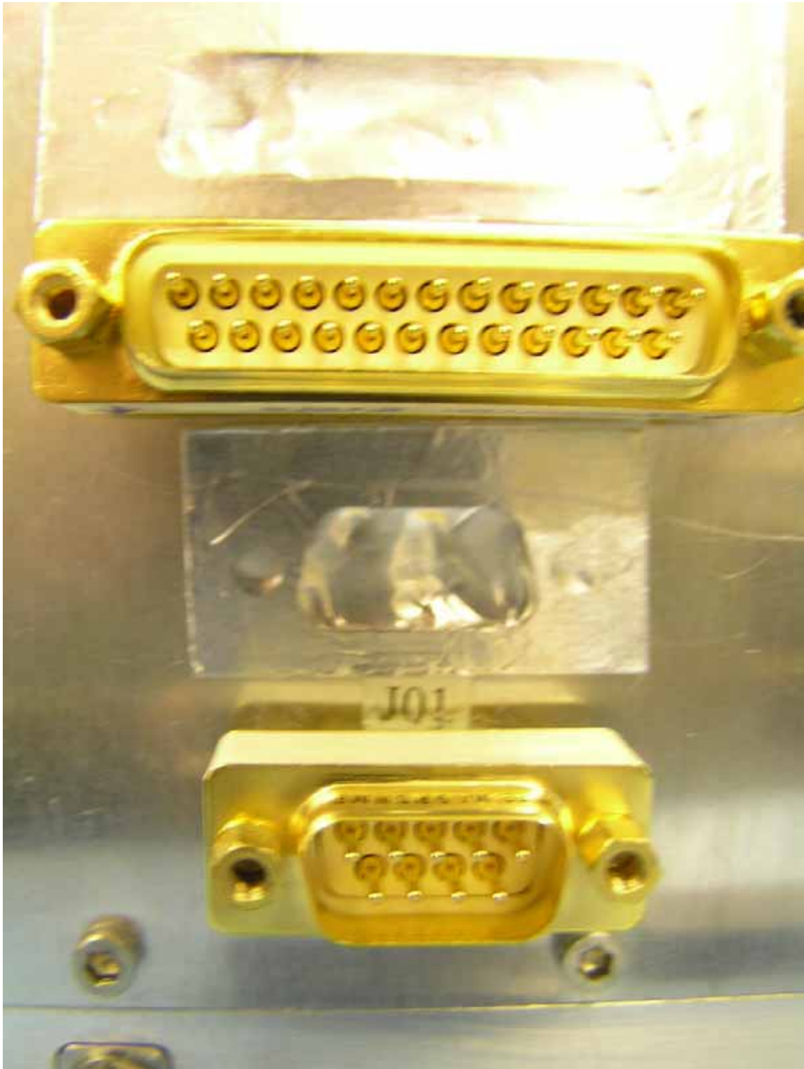
Close up of Connectors J01 & J07 with J07 ESD cover removed
