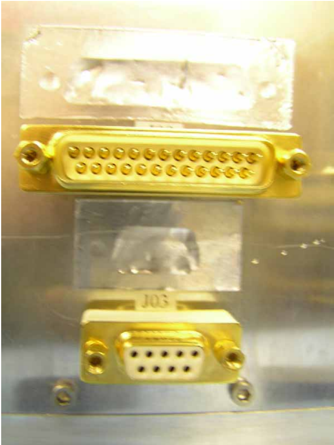
Close up of Connectors J03 & J08 with J08 ESD cover removed
