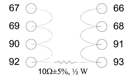
Contacts 67, 69, 90 and 92 daisy chained as indicated above Contacts 66, 68, 91 and 93 daisy chained as indicated above Contacts 92 and 93 bridged by a resistor as indicated above All other contacts left open circuit
