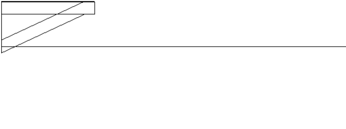
Fig. 5.3-3: Detailed view of the section between M1 (M1 rim shown on the left side) and sunshade, for the Gap Closure Model. Only the lower part of the central sunshade is shown (vertical line on right side).
