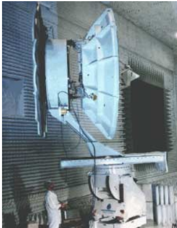
Figure 15-13 : 4m Cassini Antenna under test in the ALCATEL CATR
