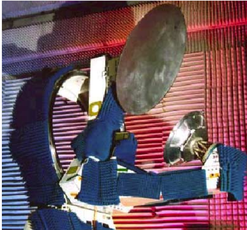
Figure 2-2 : RFDM under test configuration in CATR.
