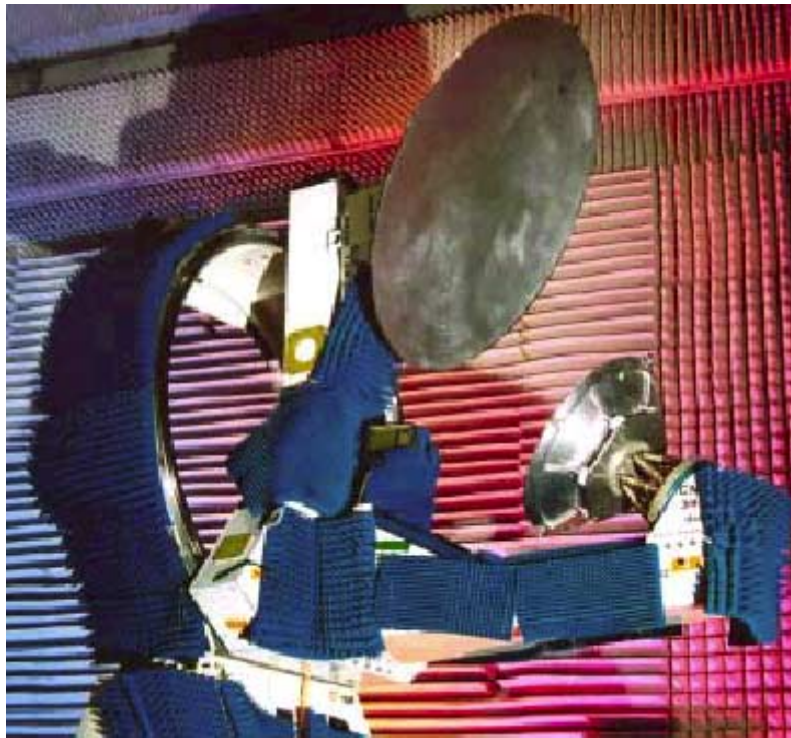
Figure 6-11 : RFDM under test configuration in CATR.
