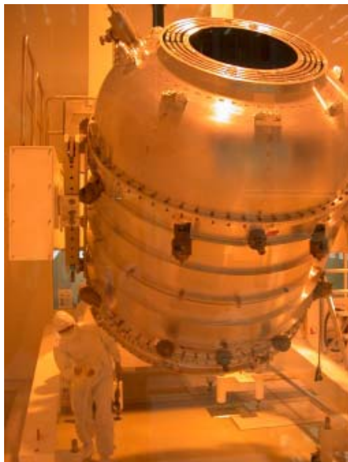
Figure 5-8: Cryostat tilted in Integration Dolly in Clean Room 100 at Astrium Ottobrunn
