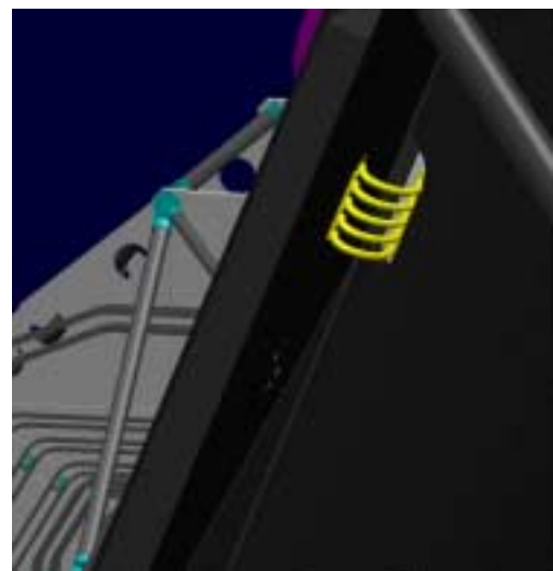
Figure 5.6-19 : Thermal braids at the rear side of the Baffle
