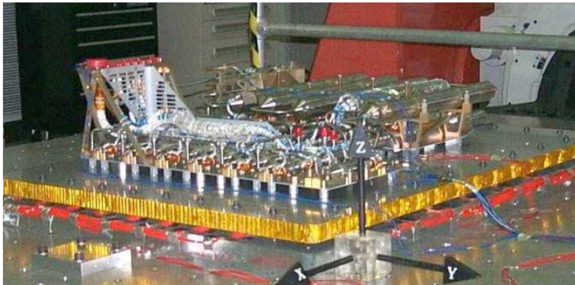
Figure 5.1-22 Sorption cooler FM1 compressor under vibration tests
