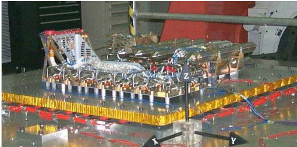
Figure 5.1-22 Sorption cooler FM1 compressor under vibration tests
