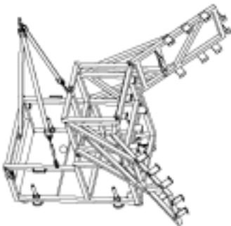
Figure 13 - SCC Panel Stiffener Device (SPSSD) on its trolley with hoisting device
