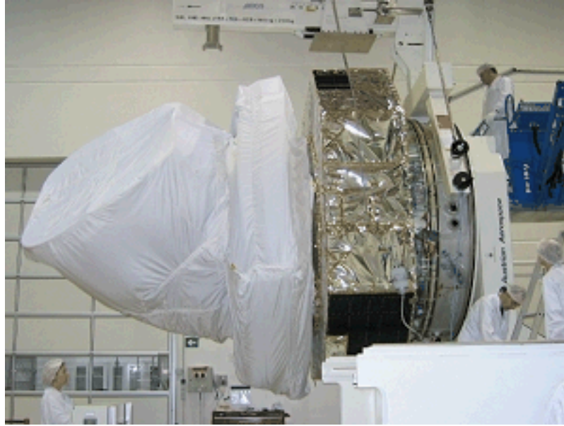
figure 19: PPLM protections for S/C transportation (COM)
