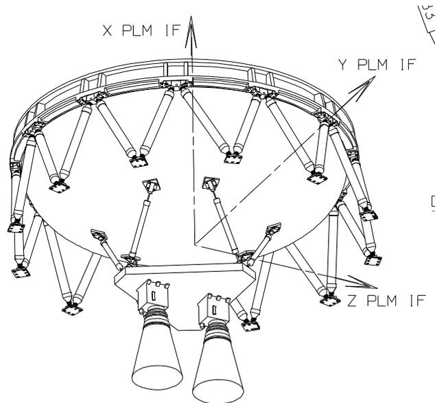
Figure 2-2 for stability reason, star trackers are interfaced to PLM , not SVM
