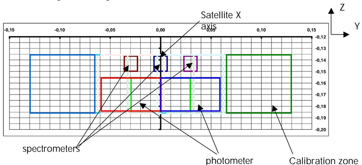
The angle between this FOV orientation and Y satellite (nominally 0deg), quantifies the PACS around LOS.
