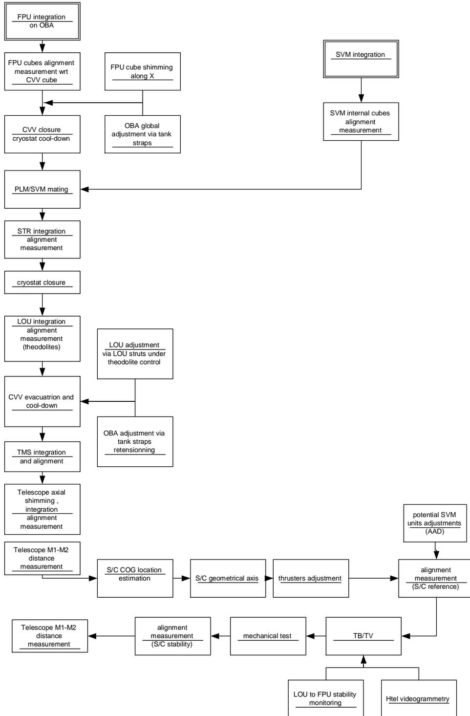
Figure 5-1 FM alignment flow
