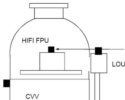
Figure 2-4 LOU to HIFI FPU coalignment - schematic
