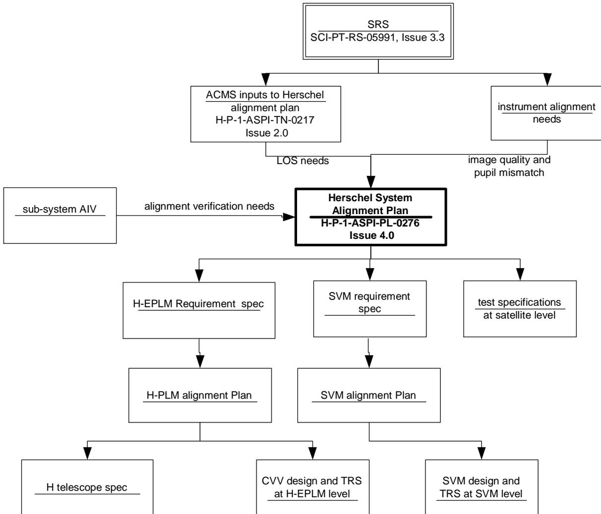
Figure 1-1 requirements flow down from SRS down to modules design
