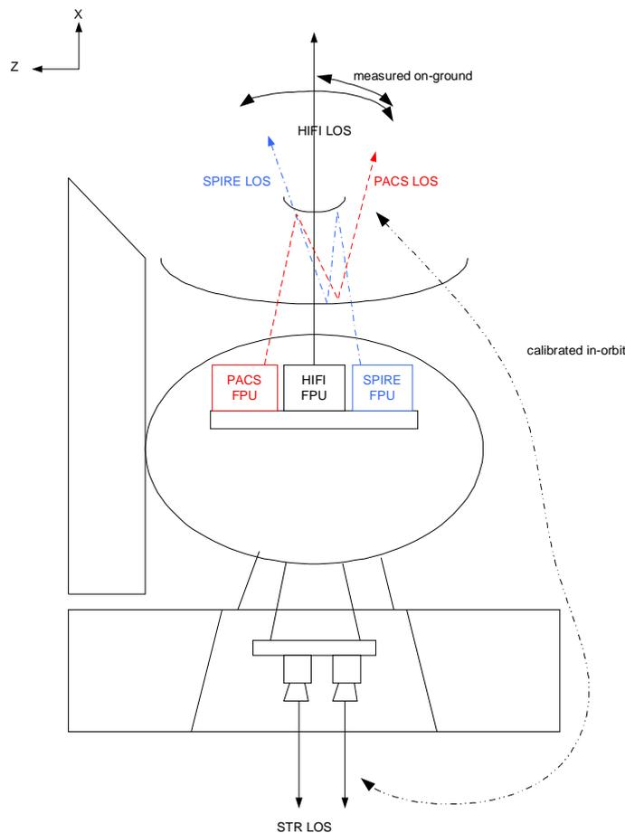
Figure 2-3 instruments LOS schematic projection on the sky
