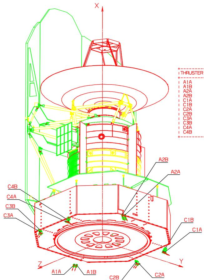
This alignment is based on classical theodolite measurements, and uses removable optical cubes located on the thruster nozzles. A 2° adjustment capability (rotations) is available on each thruster (see [RD10] thruster bracket user's manual)
