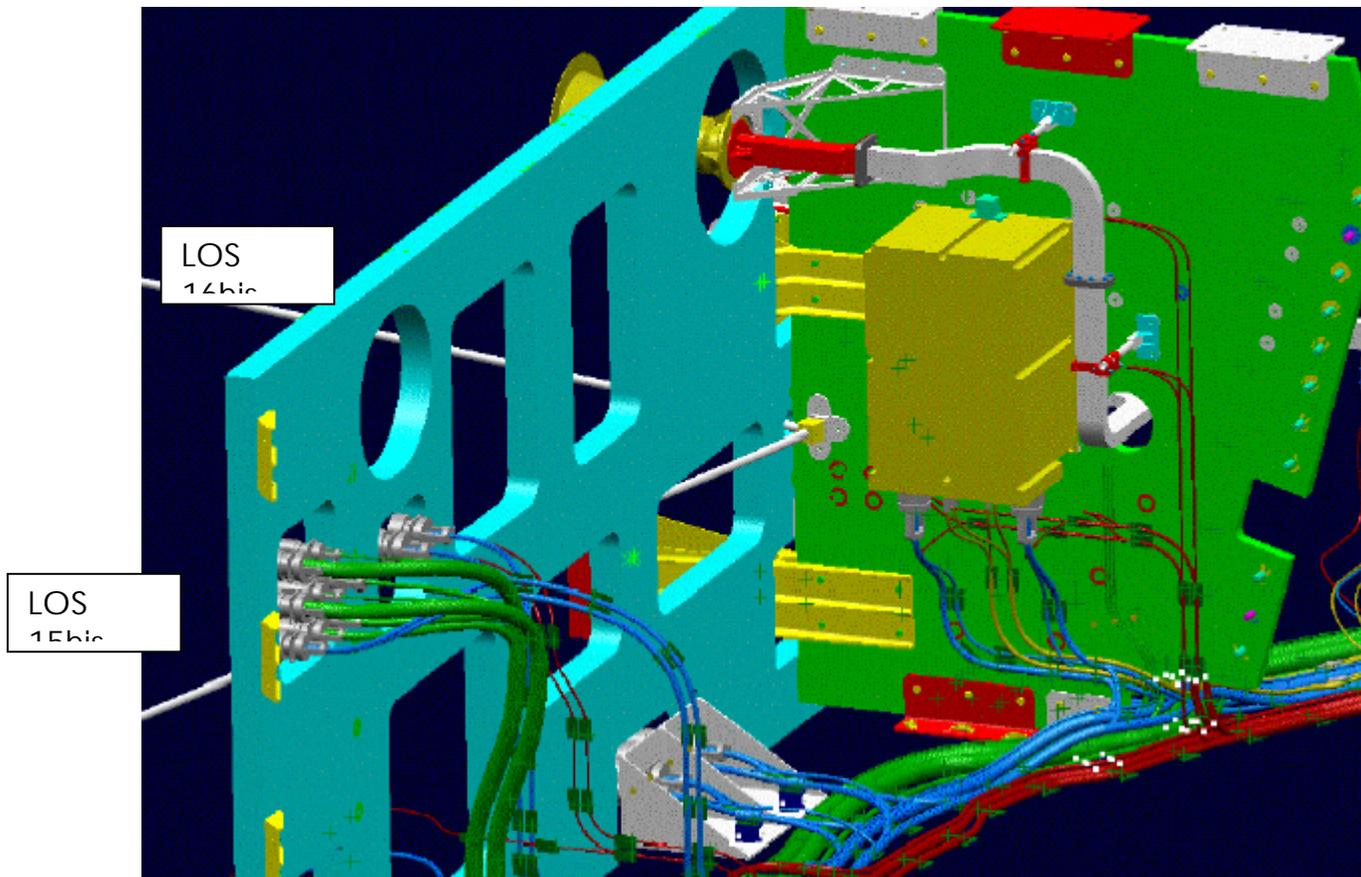
LOS 15bis and 16bis are accessible without any panel removal
