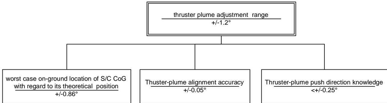
The agreed value for thruster adjustment with the RCS contractor is 2° half cone which is in line with the requirement.
