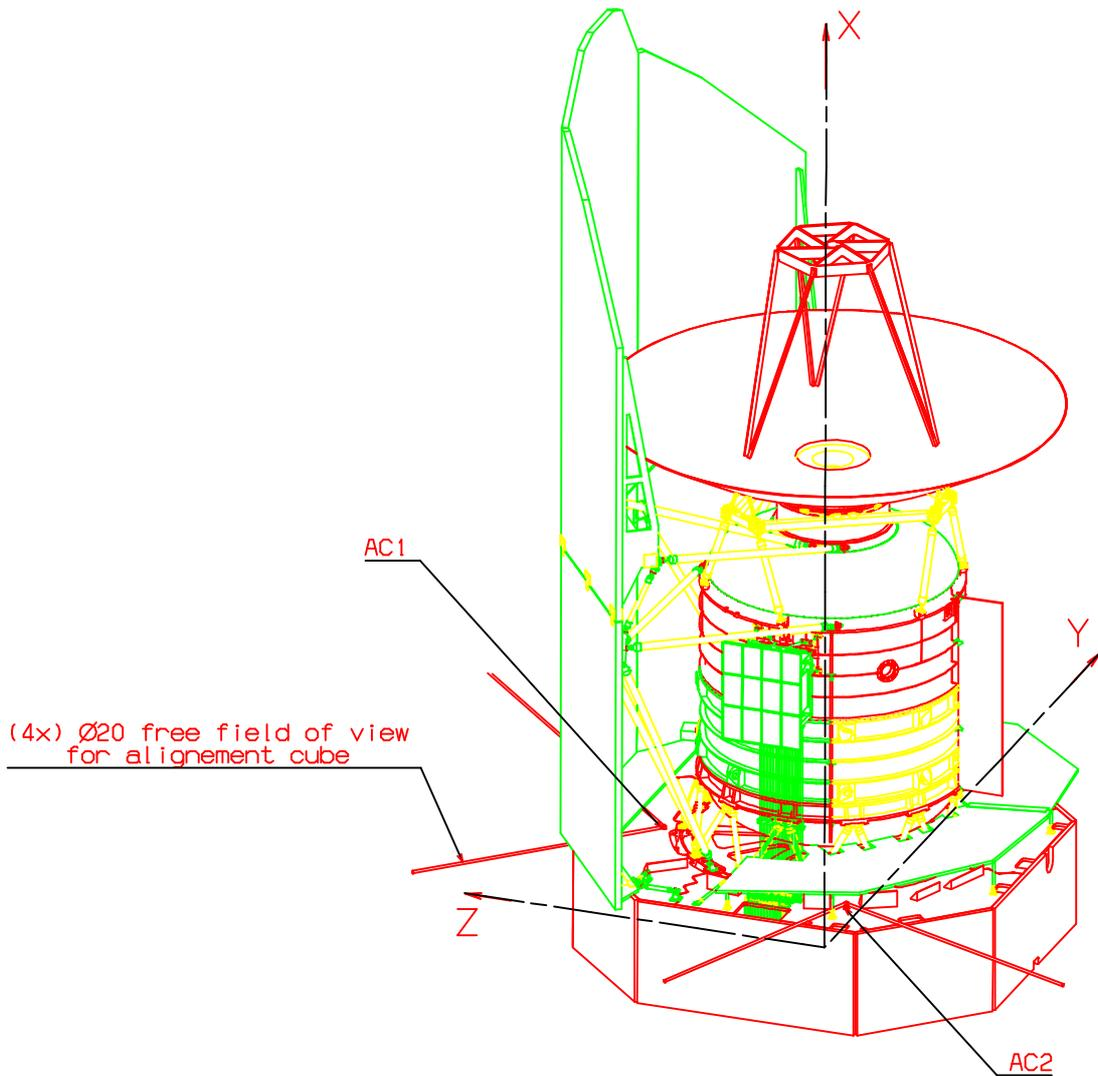
accessibility of AC1 (MRC4) at S/C level is quite difficult, so that a specific tool has been designed, as described in annex 2
