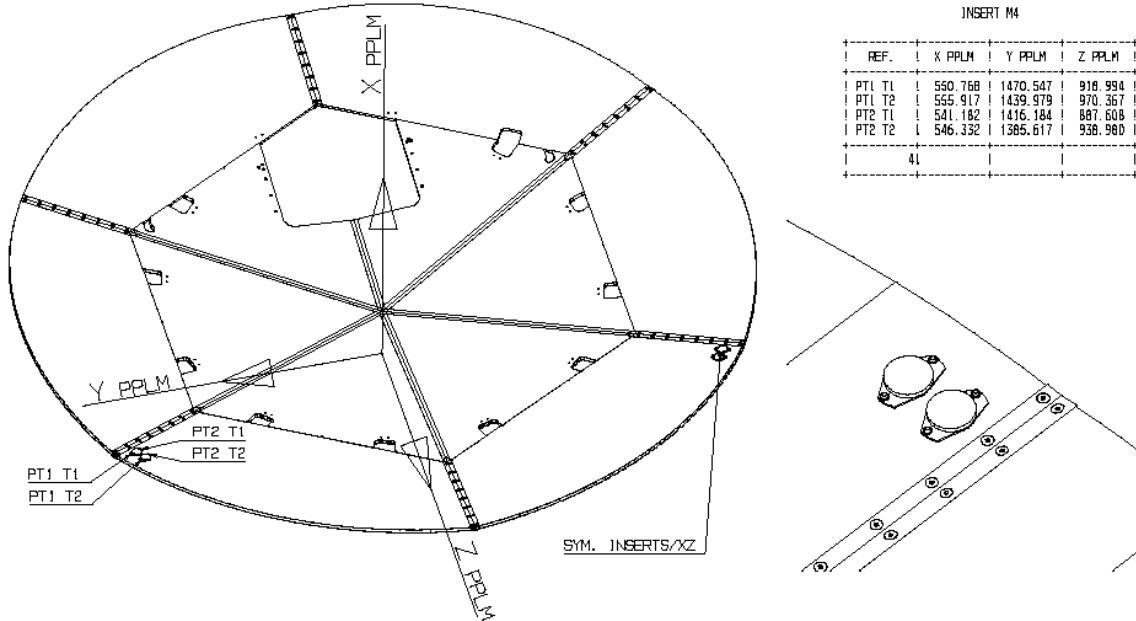
As long as the extension is not integrated, the witnesses will be put near the PPLM, to follow the parts already mounting on the flight hardware.
