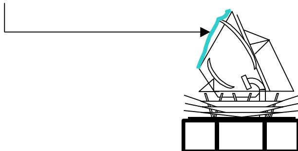
Note : this protection is linked on the PPLM baffle using velcros. The attachment points have overcome the thermal vacuum test (input check after the CQM thermal vacuum phase).
