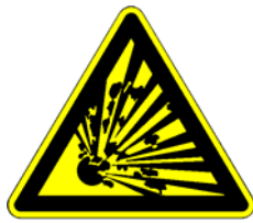
Risk of Explosion
