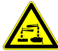
Corrosive (acid / caustic)
