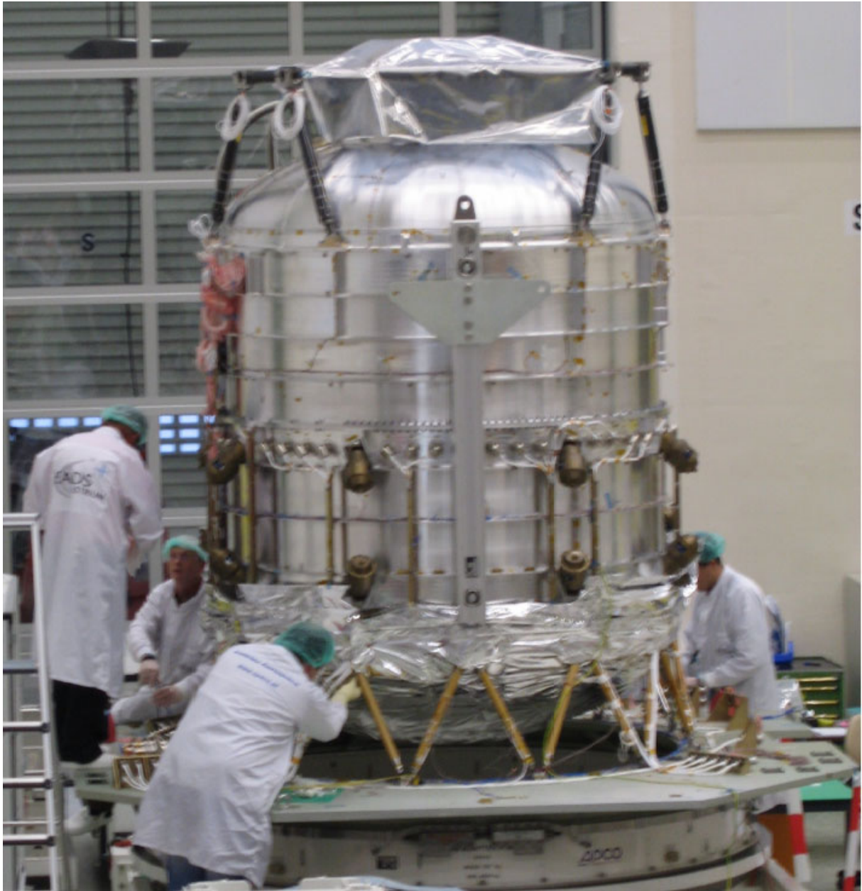
HPLM during lower bulkhead MLI integration and CVV ext. Cryo-Harness installed on TTAP.
