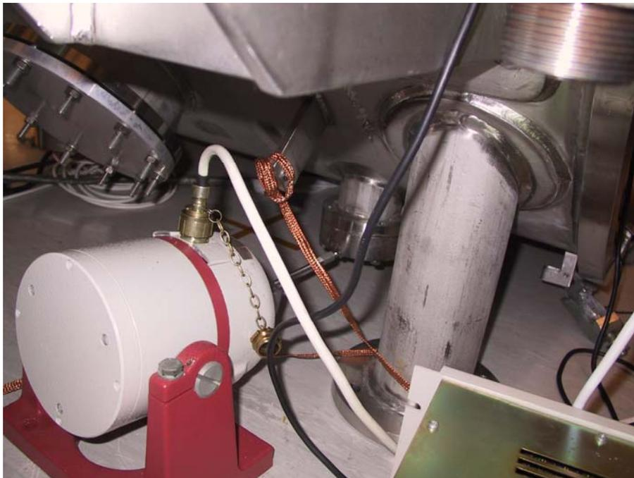
Figure 2 - Portable shaker interfacing to the chassis of the ILT cryostat
