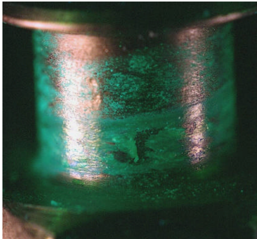
Figure 25: Unpolished pulley from previous figure under UV illumination.
