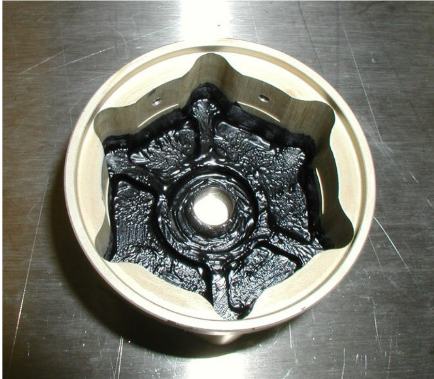
Figure 6 Preliminary inspection for integrity of black coating on cover
