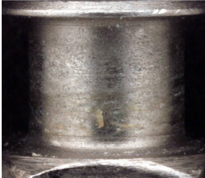
Figure 24: Unpolished pulley under visible illumination after shake-to-failure test.
