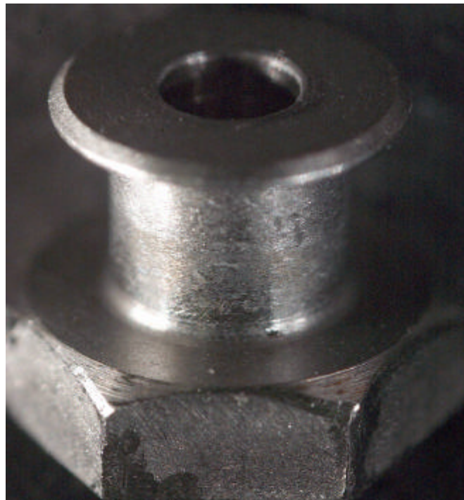
Figure 19: Unpolished pulley from Figure 18 under ordinary illumination. Kevlar debris is barely visible.
