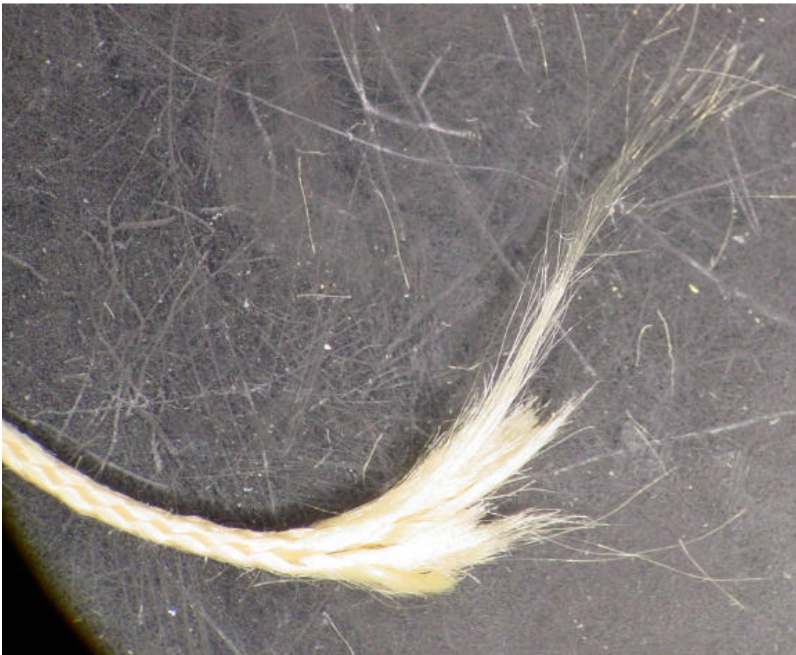
Figure 8: CQM BDA Kevlar break, Capstan-3 end.
