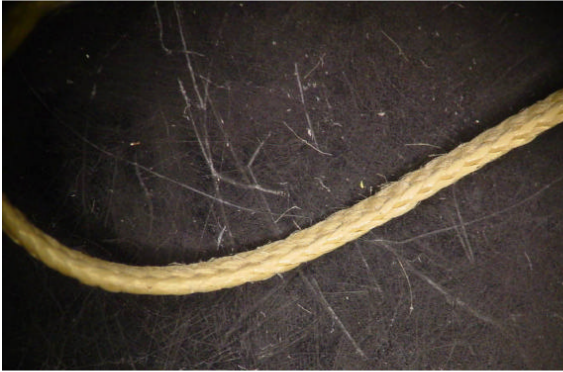
Figure 9: CQM lower braid Kevlar from pulley #2 area, showing abrasion where the Kevlar was against the pulley barrel.
