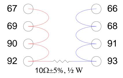
Contacts 67, 69, 90 and 92 daisy chained as indicated above Contacts 66, 68, 91 and 93 daisy chained as indicated above Contacts 92 and 93 bridged by a resistor as indicated above All other contacts left open circuit
