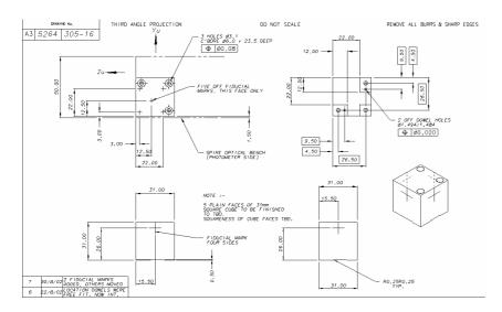
The position of the alignment cube wrt the spacecraft axis is given in the table below.
