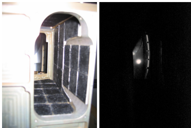
Figure 9: Looking through the FPU entrance aperture with external light to show the present geometry and features (left), and with just the back illumination from PSW position (right) to identify the stray illuminated parts
