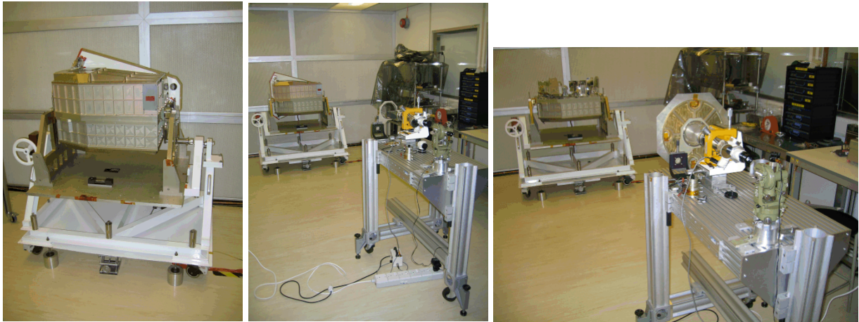
Figure 1: SPIRE FS FPU in the ambient alignment set-up (left), with the LAM M2 OGSE bench being aligned to the simulated Herschel axis optical reference (centre), and with Phot cover open and LAM M2 bench with M2 tool in position (right).
