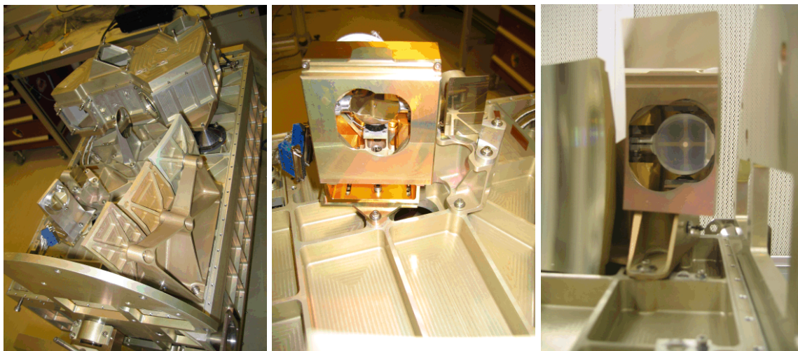
Figure 3: FS FPU Phot side with OGSE BSM (left), FS BSM mounted on SOB (centre), and view of the BSM, superimposed (with image of CS tool) through reflection in CM3 (right).
