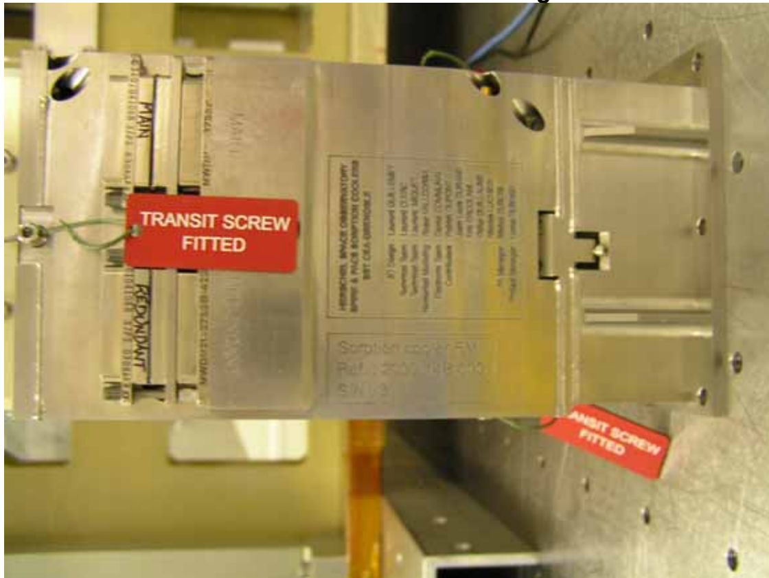
Cooler out of Pressurised Transit container showing Transit Screw 1 fitted
