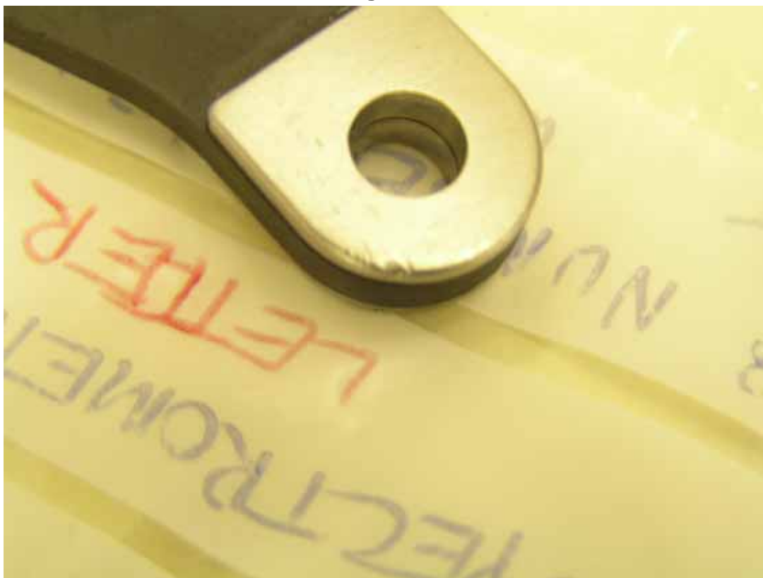
Spectrometer box A frame A showing Scratches on Metal face
