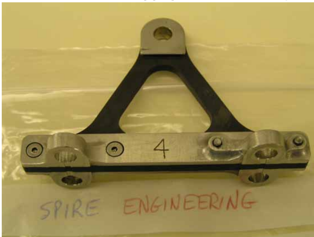
Photometer box A frame 4 showing gouge in metal surface at top
