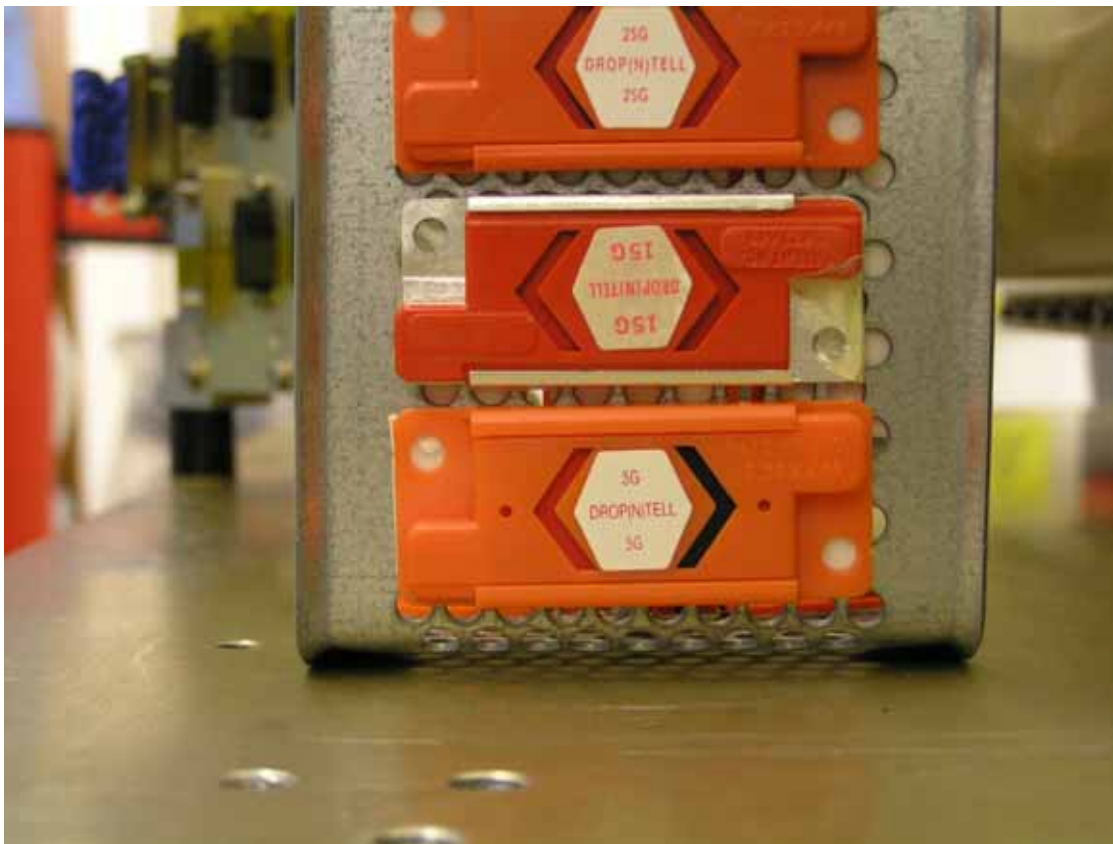
VIEW of SHOCK Monitors 25g, 15g, 5g Y axis 5g Minus Tripped.
