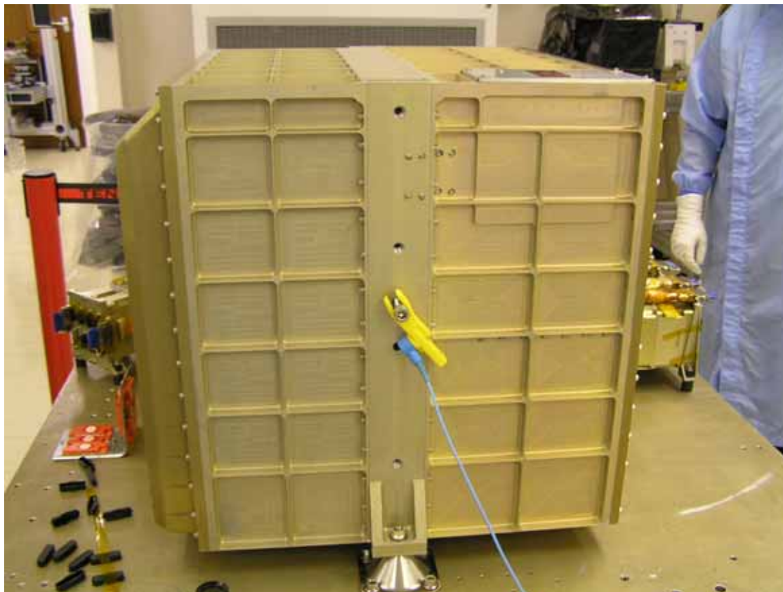
Opposite End Showing ESD strap fitted and Red Tag item Top Right
