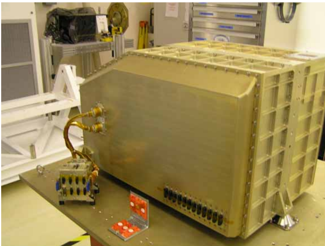
Side view showing position of Shock detectors, JFET's and ESD connector covers fitted
