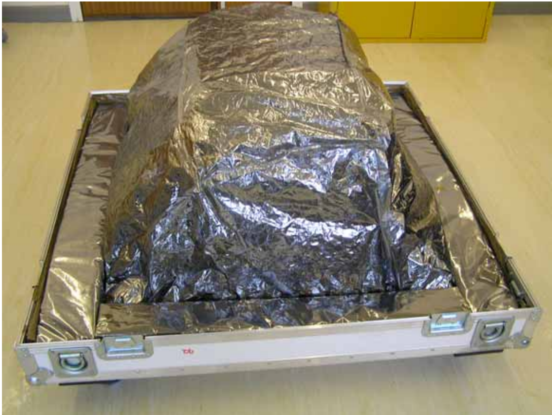
CQM on Transit container Base Triple Bagged (In Prep Area)
