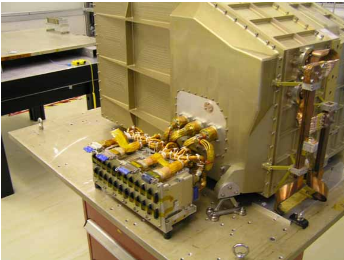
Side view showing Thermal straps & JFET's with ESD connector covers fitted
