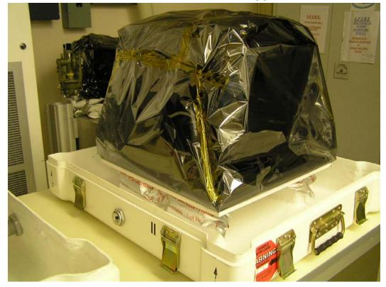
DCU and FCU – secured to case bases and double bagged.
