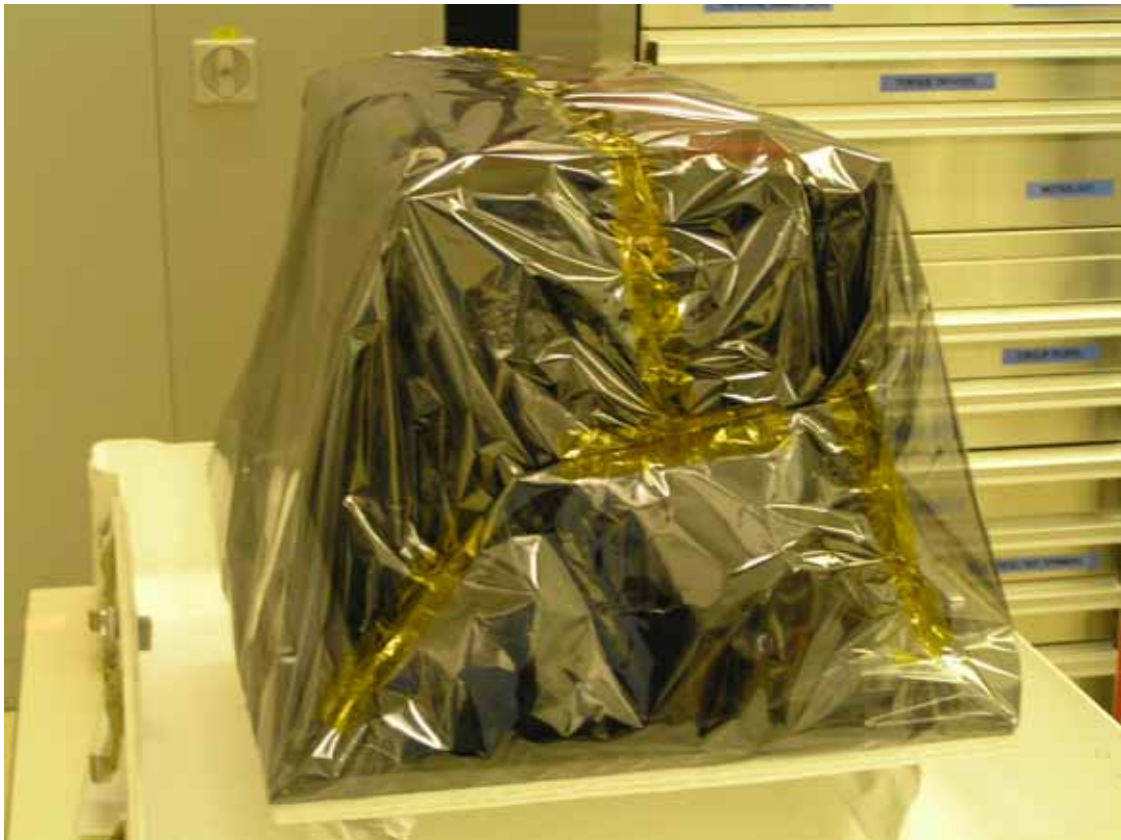
FCU Bagged ready for container lid to be fitted
