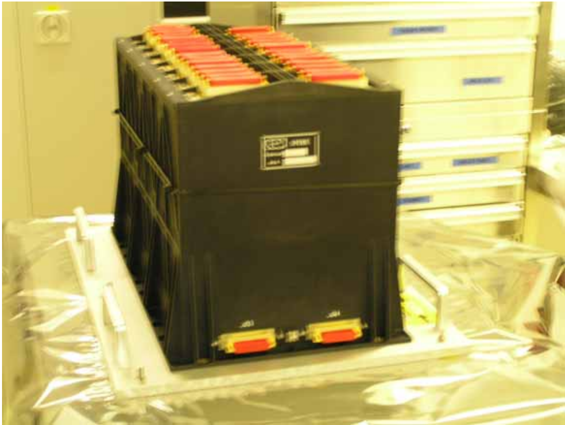
FCU mounted on Transit Plate savers and Connector covers Fitted
