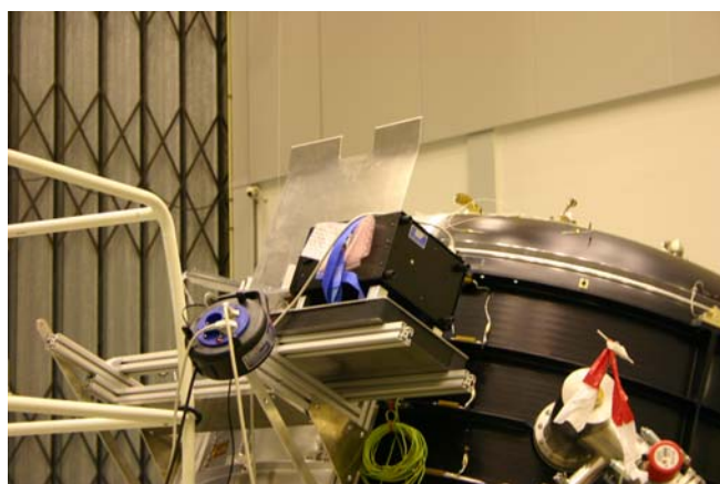
Figure 1: The external radiation source mounted on its frame on the outside of the Herschel cryostat.
