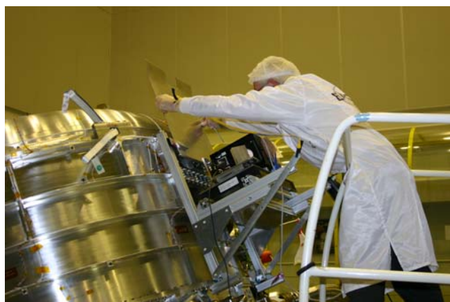
Figure 3: Removing the protective shield in front of the external source. This shield covered all LOU and alignment ports and was used to define the “on” and “off” states for the test.
