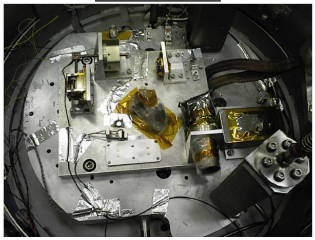
A view of the test items mounted on their vibration fixture. The control strategy implemented involved taking the average response from the two accelerometers attached to the fixture.
