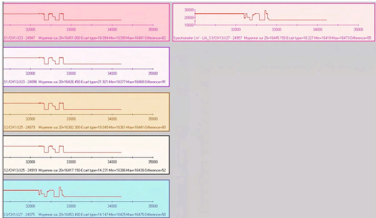
Bias level changes on every channel, discharges on BIAS-R rear connector backshell
