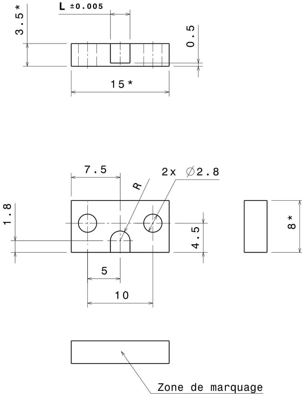
LA COTE "L" EST EGALE AU  $\varnothing$  GOUPILLE SPI-MEC-51-DD-06-A + JEU DETERMINE EN FONCTION DES MODELES
