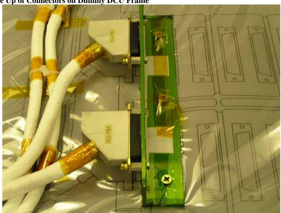
Close Up of Connectors on DCU Dummy frame
