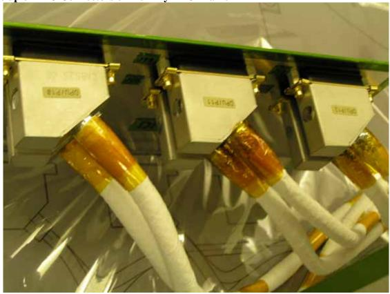
**Close Up of Connectors on Dummy DCU Frame**
