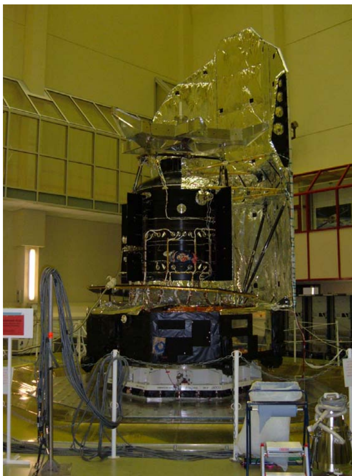
Fig. 4.1-1: Herschel S/C STM on the Hydra Shaker
