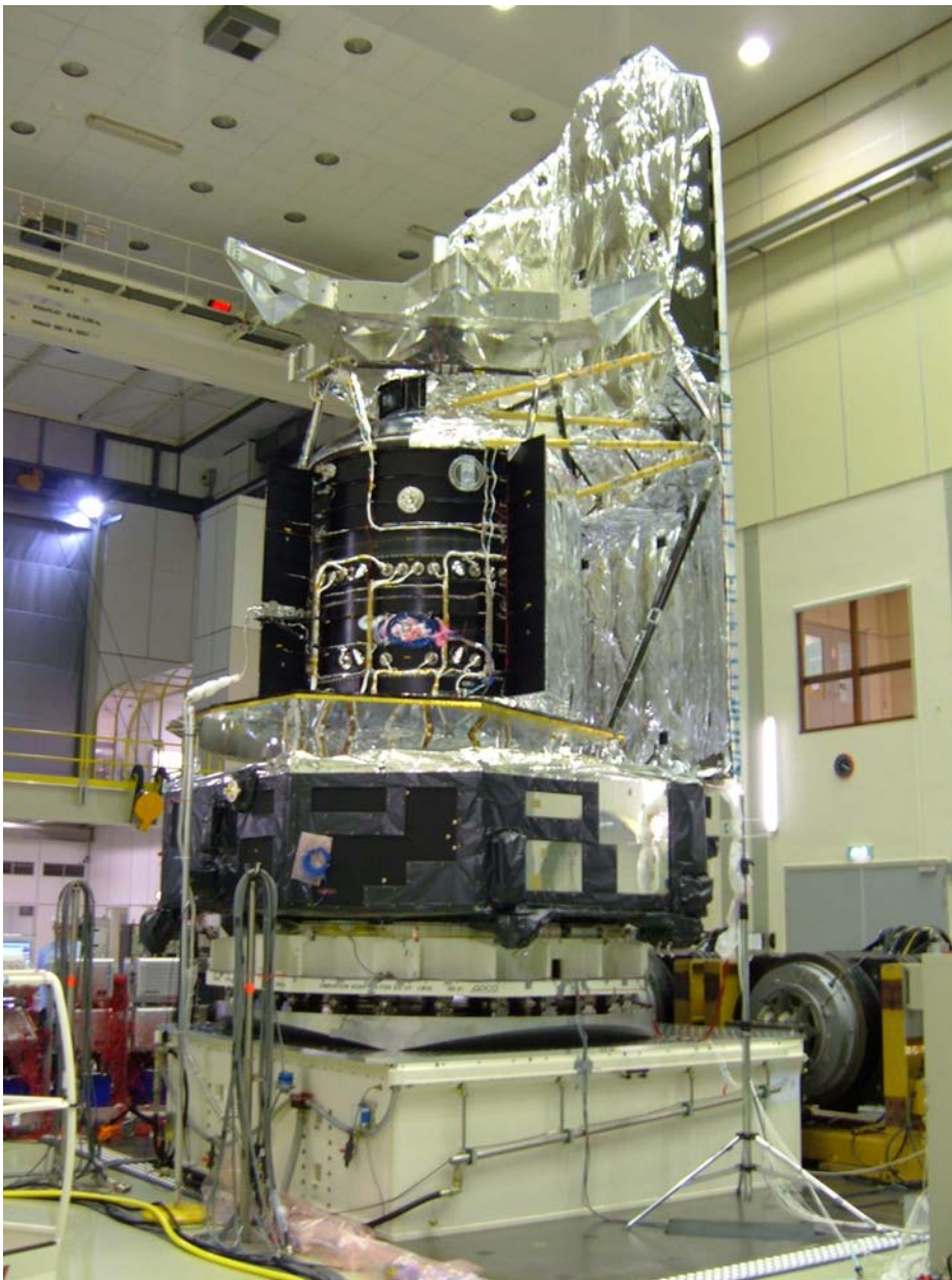
Fig. 4.2-1: Herschel S/C in Z-Axis Sine Test Configuration on Multi-Shaker
