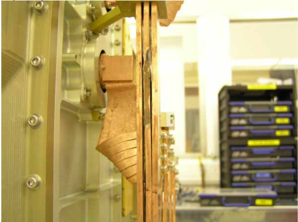
SPIRE RAL-REP-002707 issue 1 PFM out going inspection to CSL (Workmanship) Close up of Straps showing discoloration
