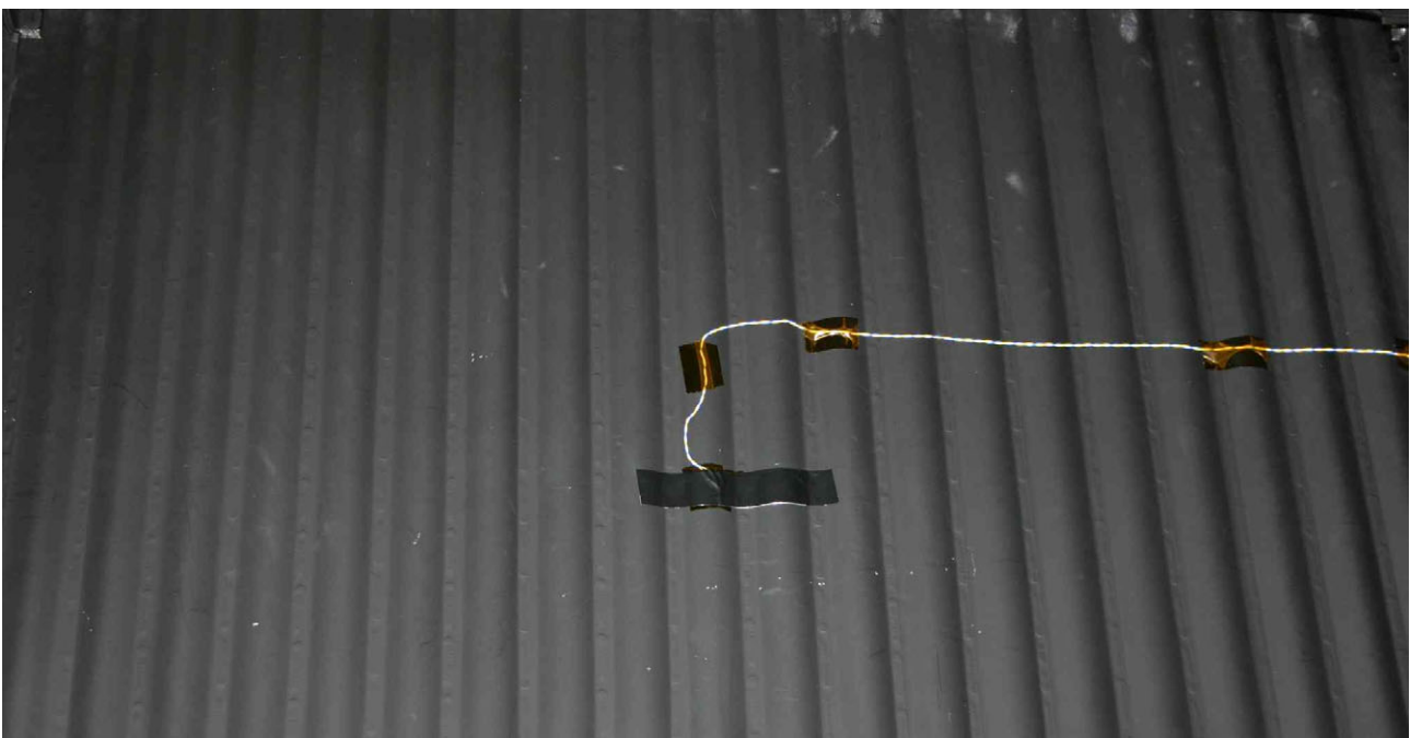
Figure 6.4-11: Typical placement of shroud temperature sensor
