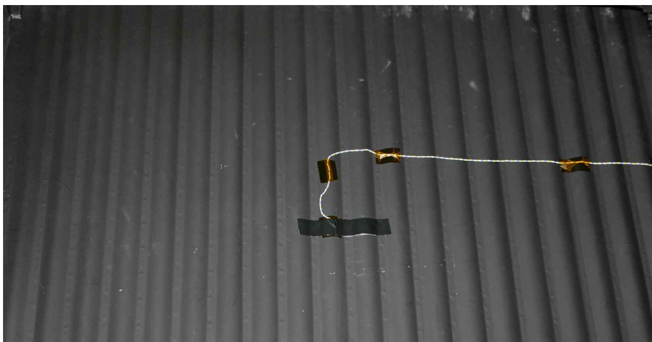
Figure 6.4-11: Typical placement of shroud temperature sensor
