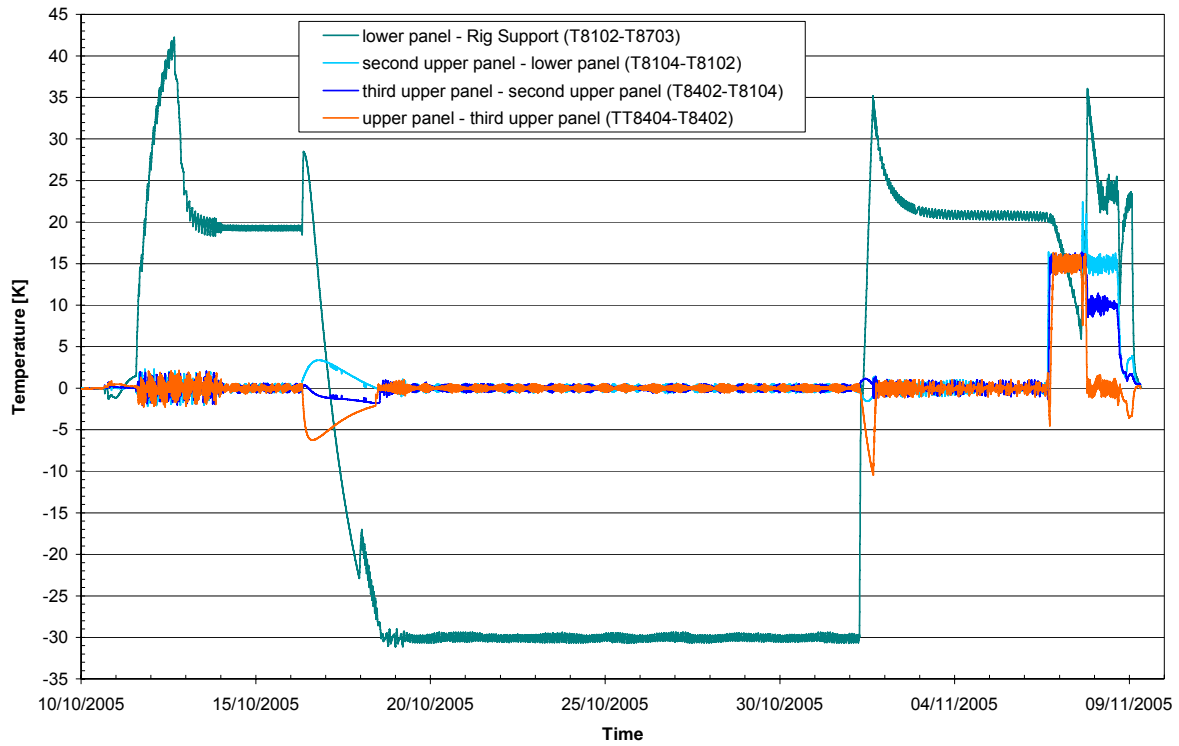
Figure 5.2-4: Temperature Gradients between IR Rig Panels and Support during all Test Phases
