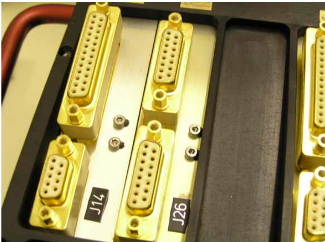
Close ups of FCU & DCU connectors with Savers Fitted
