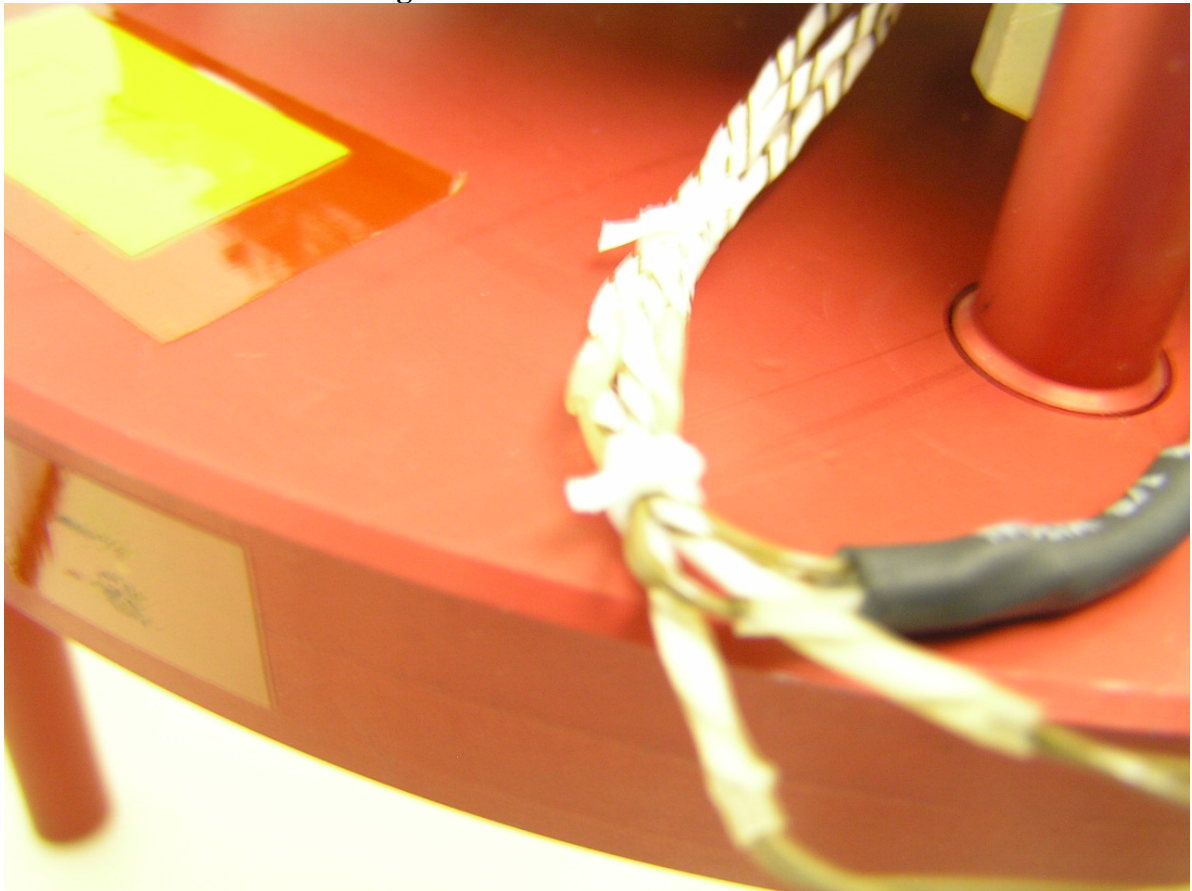
Thermistors Connected showing cable ties.
