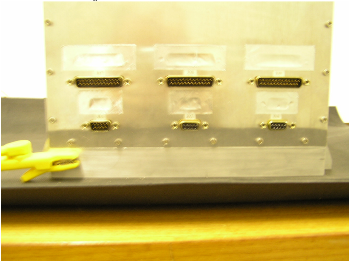
Connector Panel showing masked off redundant connector holes and ESD earth connection.
