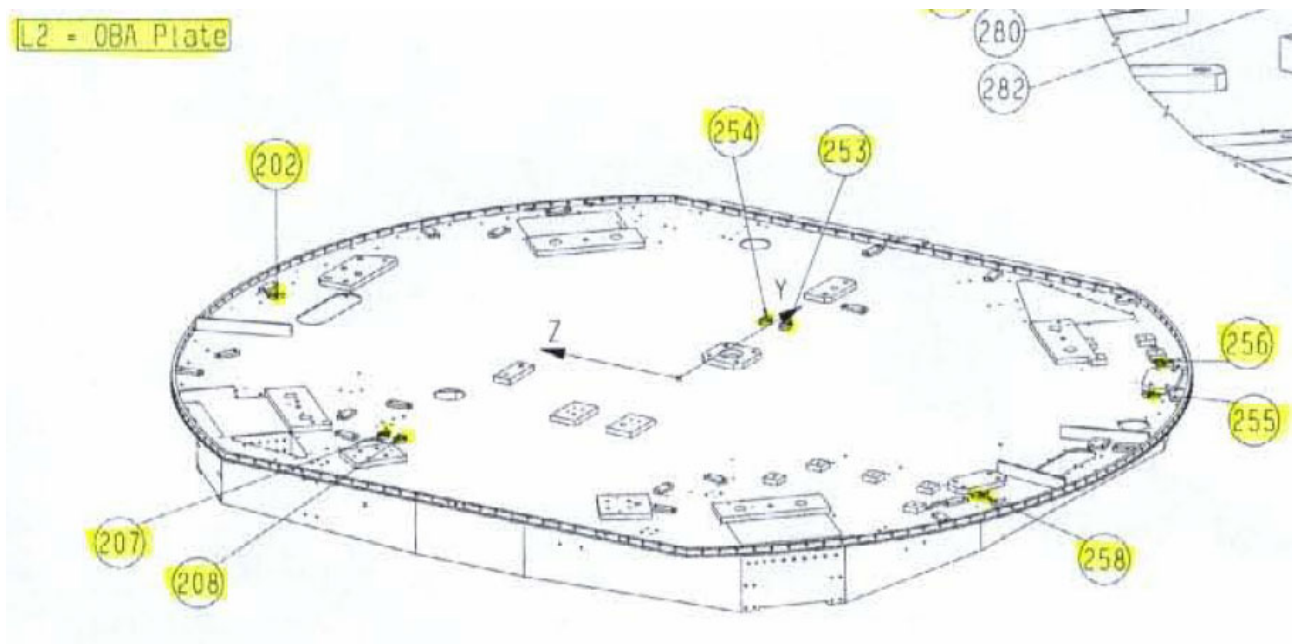
Figure 5.2-1: Distribution of Temperature Sensors on the Optical Bench Plate (L2)
