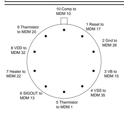
Rear view of free socket fitted to back of photo-detector block. MDM referred to is the spectrometer bias tail on C1 P10 (see Harness definition documents SPIRE-RAL-PRJ-000608 v1.1 section 4.4.1)
